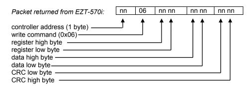
Example: Write register 60 (temperature set point) of controller at address one to 20 degrees.
