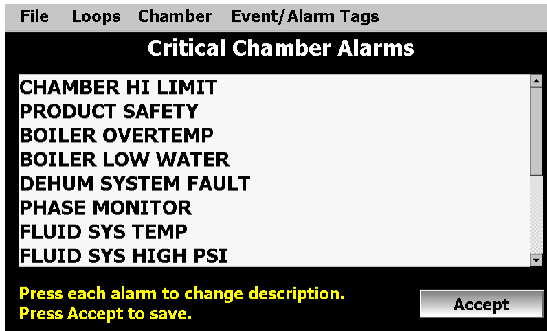
Figure 8-12 Critical Chamber Alarm Names
