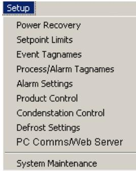
**NOTE:** Prior to entering system maintenance, all automatic chamber operations must be stopped. This includes data logging and profile operation.
