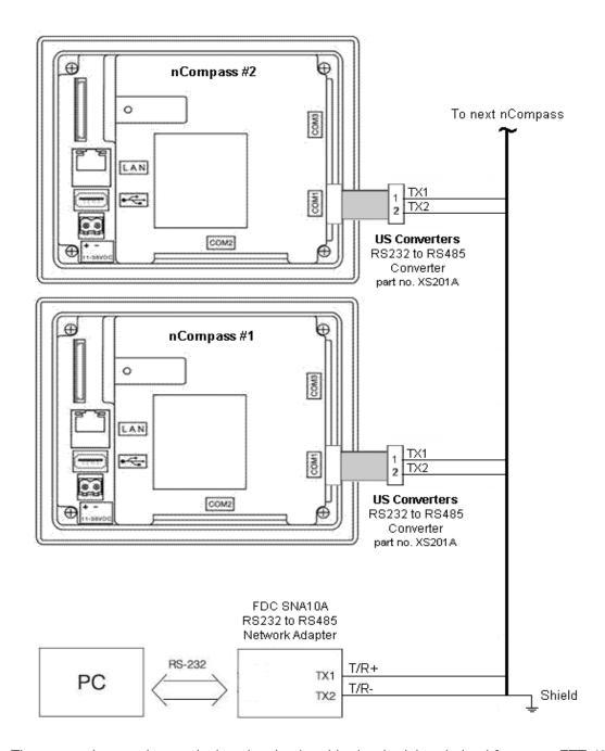
**NOTE:** The connection requires a single twisted-pair cable that is daisy-chained from one EZT-430i to the next. When using shielded twisted-pair cable, be sure to ground only when end of the cable, preferably at the RS232 to RS485 network adapter. Allowing any other portion of the cable shield to come in contact with ground, or grounding both ends, will cause ground loop currents to flow in that section of the cable which can cause communication errors.
