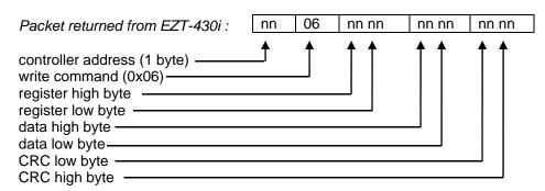
Example: Write register 41 (loop 2 set point) of controller at address one configured with no decimal point to
