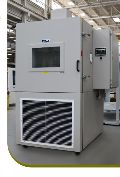
Cincinnati Sub-Zero's collaboration with the customer resulted in the successful development of a custom test chamber that meets the unique requirements for testing fuel valves. The addition of explosion-resistant features ensured that the testing environment remained secure and protected from potential ignition hazards.
