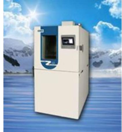
The chamber's performance will be reduced if the ambient environment where the chamber will be located exceeds 30°C. In some cases, the chamber will not operate. Condensers must be oversized to operate in high ambient room conditions.
