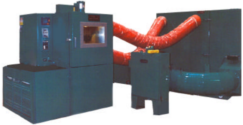
Remote conditioners are used to condition devices under test
